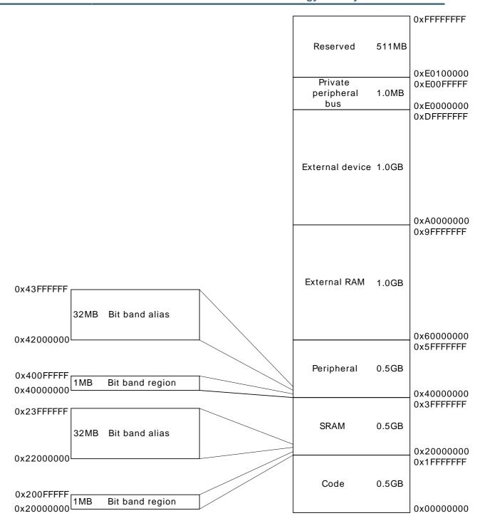
The regions for SRAM and peripherals include bit-band regions. Bit-banding provides atomic operations to bit data, see Section 2.2.5 (p. 18) .
