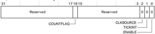
Table 4.33. SysTick CTRL register bit assignments
