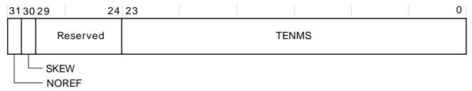
Table 4.36. CALIB register bit assignments
