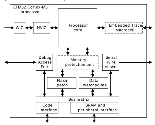
The Cortex-M3 processor is built on a high-performance processor core, with a 3-stage pipeline Harvard architecture, making it ideal for demanding embedded applications. The processor delivers exceptional power efficiency through an efficient instruction set and extensively optimized design, providing highend processing hardware including single-cycle 32x32 multiplication and dedicated hardware division.
