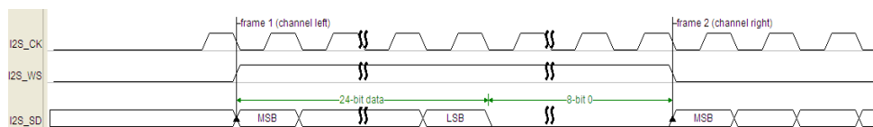
Figure 15-20 MSB justified standard timing diagram (DTLEN=01, CHLEN=1, CKPL=1)
