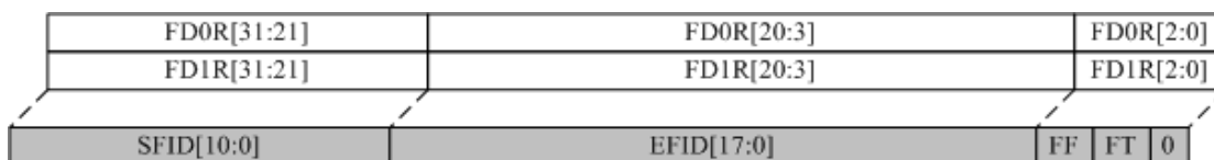
Figure 21-8 32-bit list mode filter
