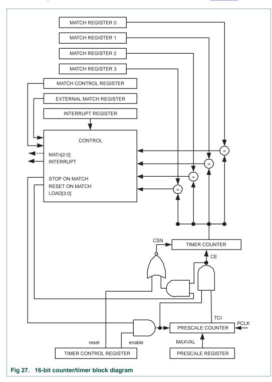
The block diagram for counter/timer0 and counter/timer1 is shown in Figure 27.
