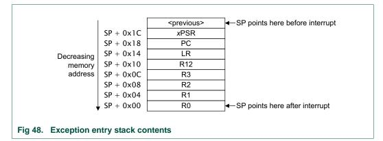
Immediately after stacking, the stack pointer indicates the lowest address in the stack frame. The stack frame is aligned to a double-word address.
