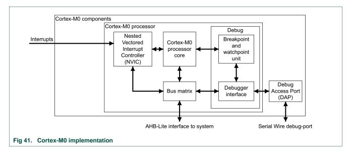
The Cortex-M0 processor is built on a highly area and power optimized 32-bit processor core, with a 3-stage pipeline von Neumann architecture. The processor delivers exceptional energy efficiency through a small but powerful instruction set and extensively optimized design, providing high-end processing hardware including a single-cycle multiplier.
