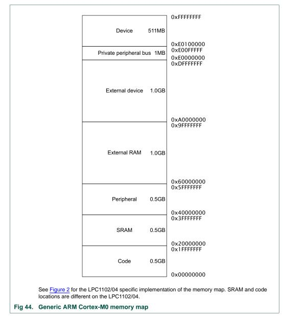
The processor reserves regions of the **Private peripheral bus** (PPB) address range for core peripheral registers, see <u>Section 19–19.2</u>.
