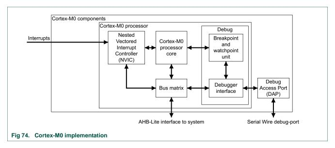
The Cortex-M0 processor is built on a highly area and power optimized 32-bit processor core, with a 3-stage pipeline von Neumann architecture. The processor delivers exceptional energy efficiency through a small but powerful instruction set and extensively optimized design, providing high-end processing hardware including a single-cycle multiplier.
