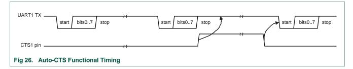
During transmission of the second character the  $\overline{\text{CTS}}$  signal is negated. The <u>third</u> character is not sent thereafter. The USART maintains 1 on TXD as long as  $\overline{\text{CTS}}$  is negated (high). As soon as  $\overline{\text{CTS}}$  is asserted, transmission resumes and a start bit is sent followed by the data bits of the next character.
