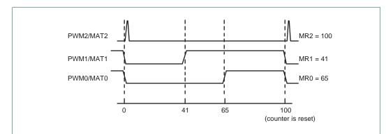
Fig 56. Sample PWM waveforms with a PWM cycle length of 100 (selected by MR2) and MAT2:0 enabled as PWM outputs by the PWMC register.
