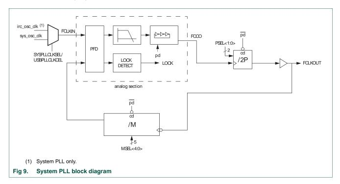
The block diagram of this PLL is shown in Figure 9. The input frequency range is 10 MHz to 25 MHz. The input clock is fed directly to the Phase-Frequency Detector (PFD). This block compares the phase and frequency of its inputs, and generates a control signal when phase and/ or frequency do not match. The loop filter filters these control signals and drives the current controlled oscillator (CCO), which generates the main clock and
