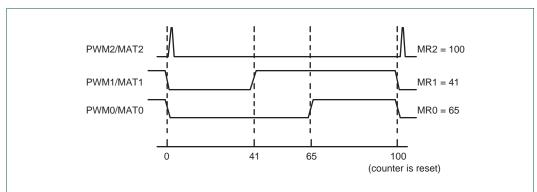
Fig 60. Sample PWM waveforms with a PWM cycle length of 100 (selected by MR2) and MAT2:0 enabled as PWM outputs by the PWMC register.
