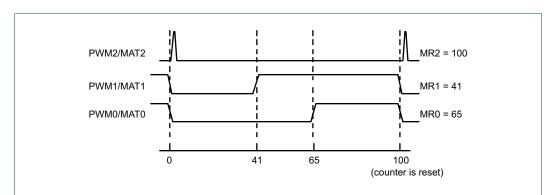
Fig 74. Sample PWM waveforms with a PWM cycle length of 100 (selected by MR2) and MAT2:0 enabled as PWM outputs by the PWMC register.
